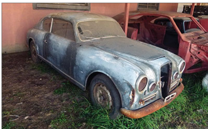
This ultra rare Lancia B20 coupe was spotted at Shawn Tyler's scrap yard on the old Pretoria-Benoni road near Petit. Body is aluminium, engine is a narrow-angle V6.
