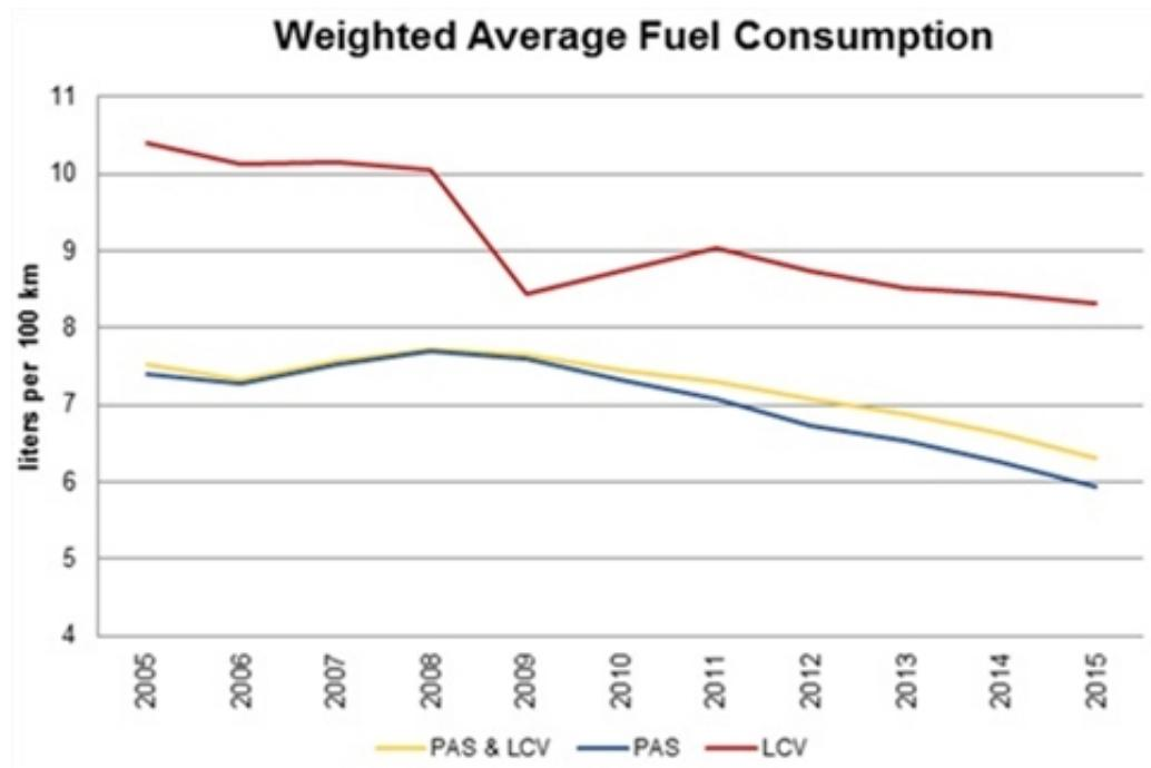
In 2006, the weighted average fuel consumption of passenger (PAS) vehicles was at 7.19 litres per 100km, and in August 2015 that number dipped to 5.86 litres per 100km. Light commercial vehicles (LCV) average fuel consumption in 2006 was 10.3 litres per 100km, and in 2015 this decreased to 8.42 litres per 100km.
